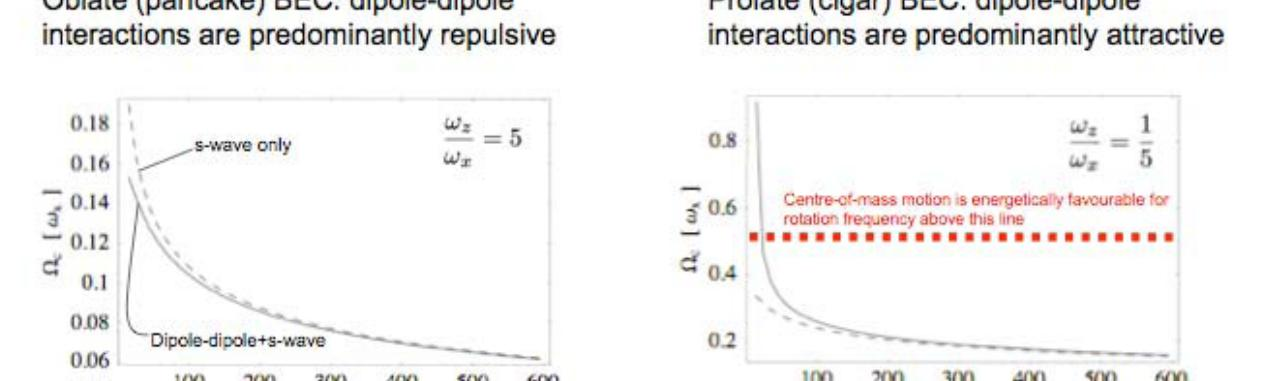
Energy for centre-of-mass motion having angular momentum L=n\hbar/2\pi is  $E_{com}^{L=1} = \frac{1}{2} N m \omega_z^2 \epsilon_{dd}^2 = \frac{1}{2} N \hbar \omega_z$
