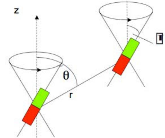
$$B(t) = B_0 [\cos(\varphi) \hat{z} + \sin(\varphi) \{ \cos(\Omega t) \hat{x} + \sin(\Omega t) \hat{y} \}] \Rightarrow \langle U_{dd} \rangle_i = \frac{\mu_0 \mu^2}{4\pi} \left( \frac{3 \cos^2 \varphi - 1}{2} \right) \frac{1 - 3 \cos^2 \theta}{r^3}$$
