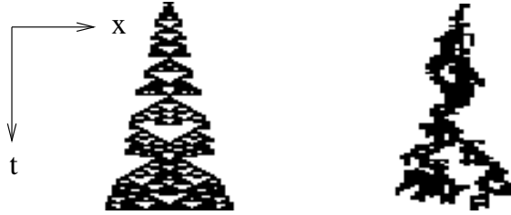
Fig. 31: Spreading process in a coupled map lattice for r = 3 and D = 0.57 . Chaotic and laminar sites are represented by black and white pixels, respectively. Deterministic synchronous updates lead to symmetric clusters (left) with nonuniversal behavior. Asynchronous updates (right) destroy these correlations, leading to typical DP clusters.
